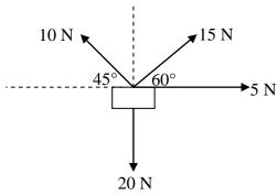
6. Both diagrams below show a particle in equilibrium under the action of various forces. In each case find the values of the unknown forces and angles.
