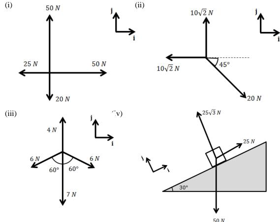
5. The diagram shows four forces acting on a package. Find the resultant force on the package.
